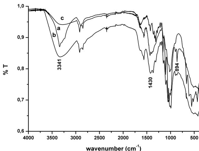
**Figure 3.** FTIR spectra of original and treated celluloses. a: FITR analysis of Bacterial cellulose, b: FITR analysis of Bacterial cellulose treated with sodium hydroxide solution at 30% in water and c: FITR analysis of Bacterial cellulose treated with sodium hydroxide solution at 30% in isopropyl
