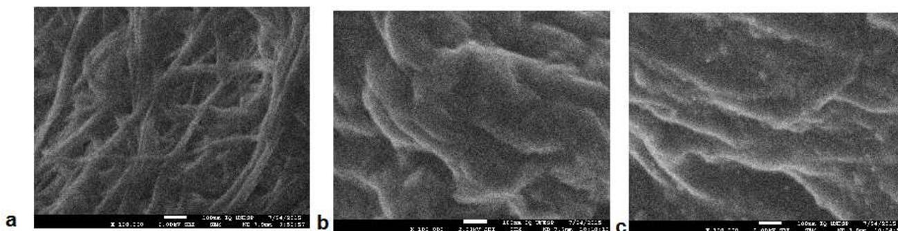
**Figure 4.** Results of analysis by scanning electron microscopy. a: Bacterial cellulose; b: Bacterial cellulose treated with sodium hydroxide solution at 30% in water and c: Bacterial cellulose treated with sodium hydroxide solution at 30% in isopropyl
