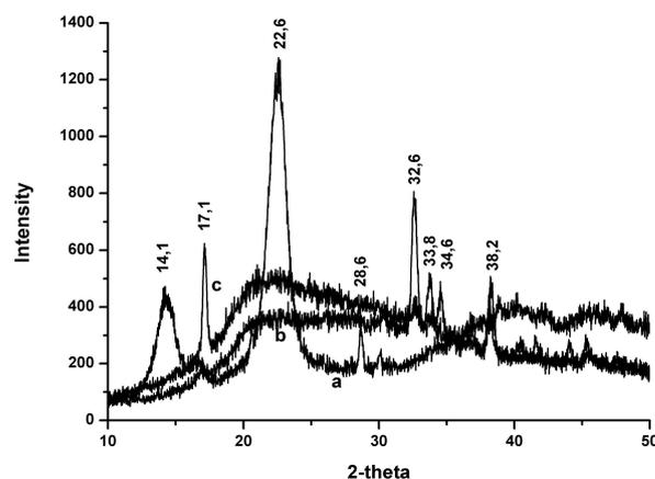
**Figure 2.** X-ray diffractogram. a: Rx analysis of Bacterial cellulose, b: Rx analysis of Bacterial cellulose treated with sodium hydroxide solution at 30% in water and c: Rx analysis of Bacterial cellulose treated with sodium hydroxide solution at 30% in isopropyl
