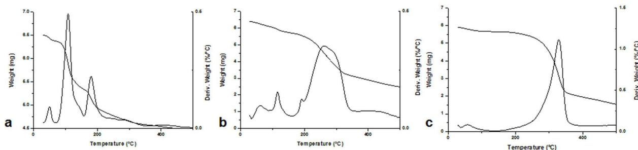
**Figure 1.** Results of thermal analysis. a: TG analysis of Bacterial cellulose; b: TG bacterial cellulose treated with sodium hydroxide solution at 30% in water and c: TG bacterial cellulose treated with sodium hydroxide solution at 30% in isopropyl
